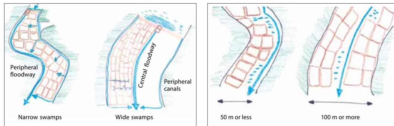
Fig. 12 Selection for Positioning of Floodway: Peripheral or Central
