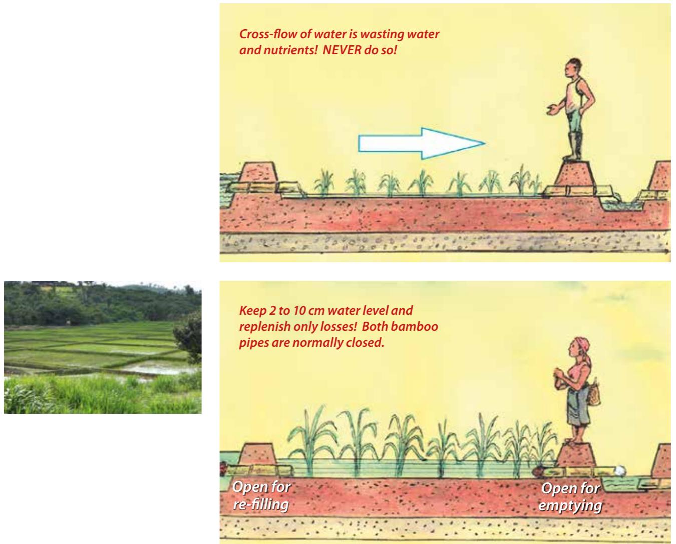
Fig. 33 Water lever regulation: constant water level in plots required
