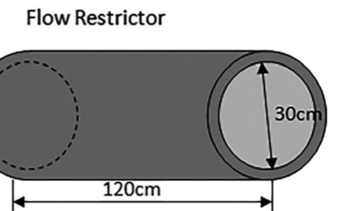
This small culvert with inner diameter 30cm is placed at the intakes in the headdike to restrict how much water goes into the field for irrigation
