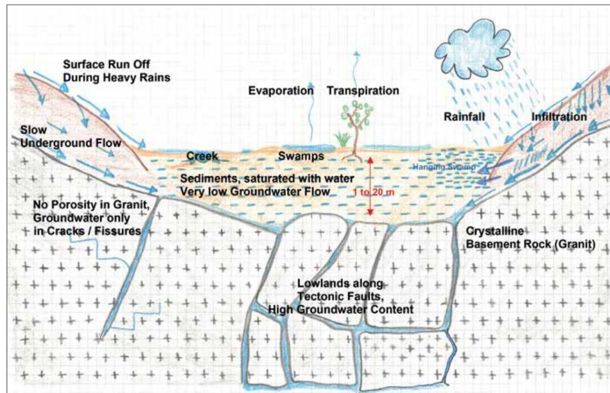
Fig. 4 Cross Profile of Lowland with Surface and Underground Flow of Water
