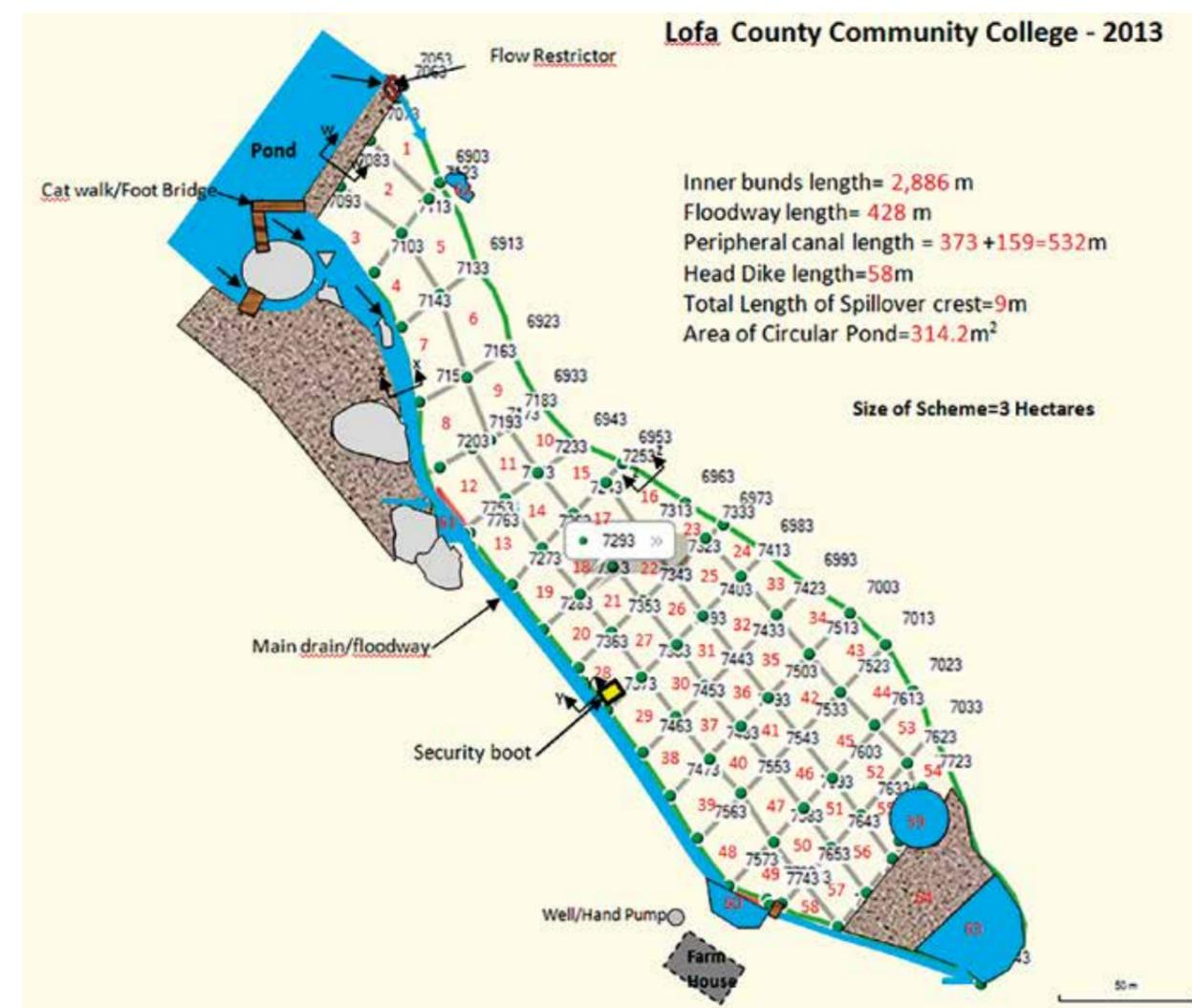
Fig. 13 A detailed swamp layout prepared with the help of a GPS data inserted into Google Earth image
