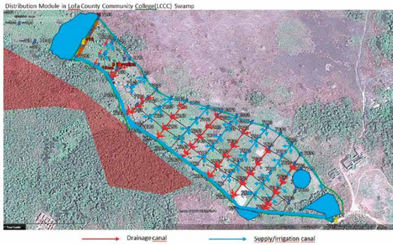
Fig. 14 A lay-out prepared with a print-out from Google Earth and hand-drawings with color pens
