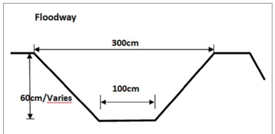
Fig. 20b Dimensions of floodways
