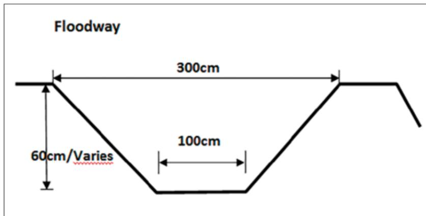
Fig. 20b Dimensions of floodways
