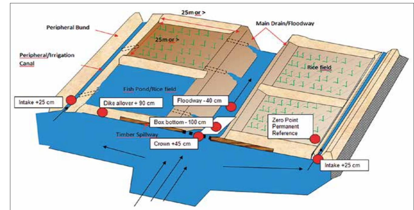
Fig. 10 Critical Levels at Head Dike and Intakes to Peripheral Canals
