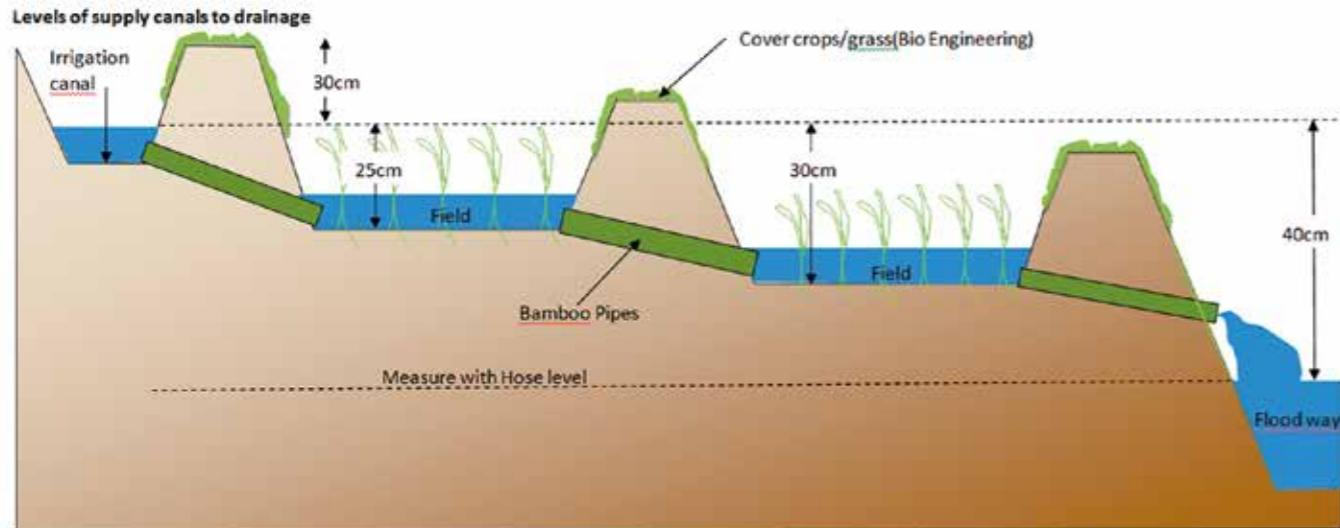
Fig. 11 Levels and Drops between Peripheral Canal and Floodway
