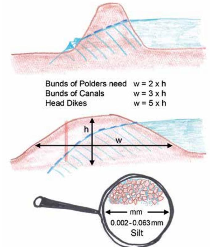
Fig. 22 Dimension of head-dikes
