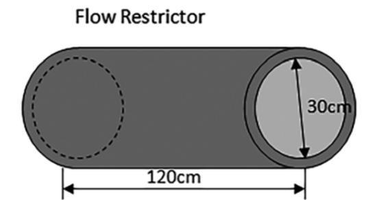
This small culvert with inner diameter 30cm is placed at the intakes in the headdike to restrict how much water goes into the field for irrigation
