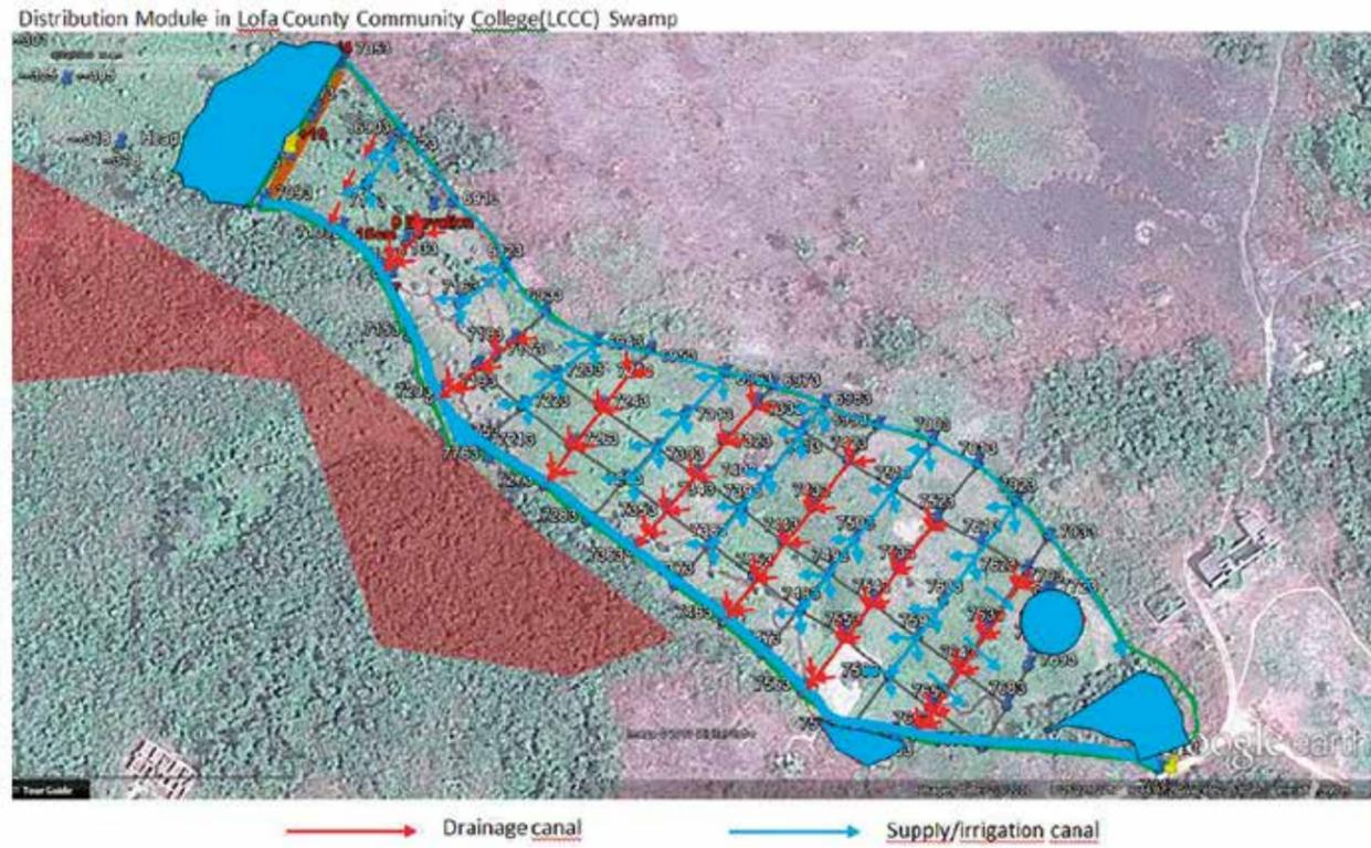
Fig. 14 A lay-out prepared with a print-out from Google Earth and hand-drawings with color pens
