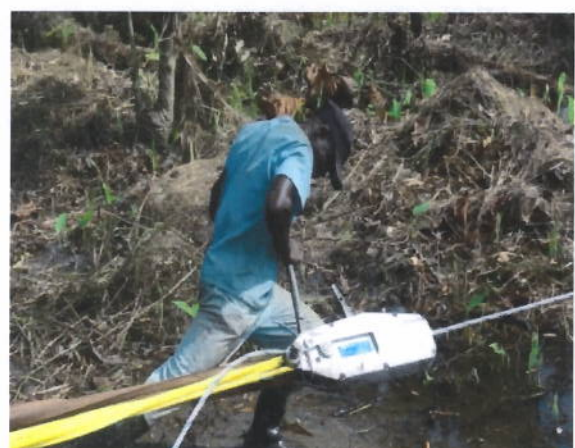
Using 'Come-A-Long' for destumping
